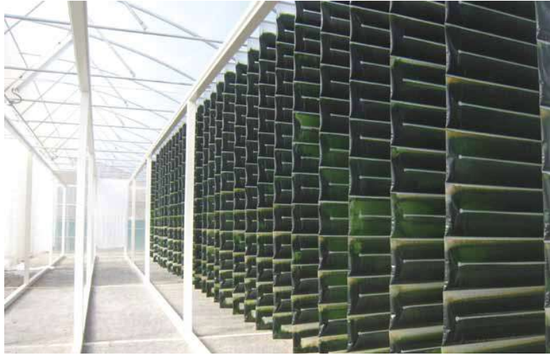
Figure 5.5 Polyethylene Sleeves for Microalgae Production (Source: Valcent Products Inc.)
