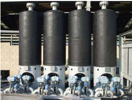
Figure 8.4 Pressure Swing Absorption System (courtesy of Tetra Tech)
