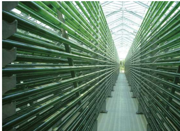
Figure 5.6 an Outdoor Tubular PBR System for Microalgae Propagation (Source: Bioprodukte-steinberg.de)
