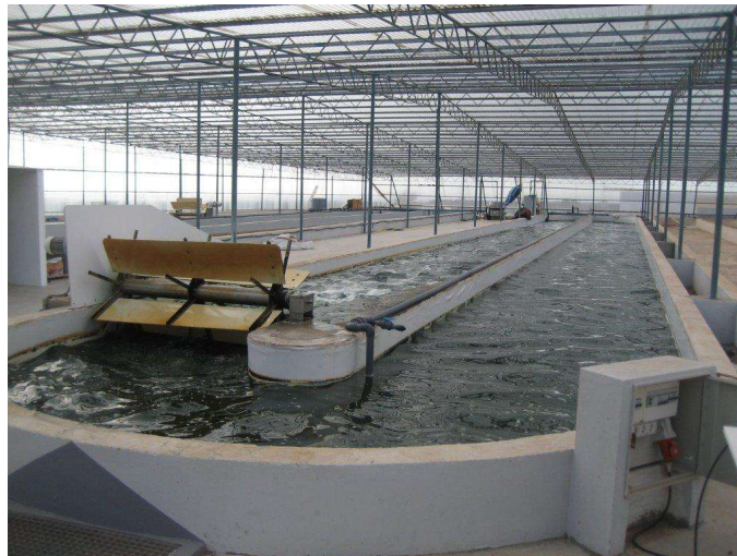
Figure 5. 2 Example of a Raceway Algae Pond (Source: NEAtech, LLC )
